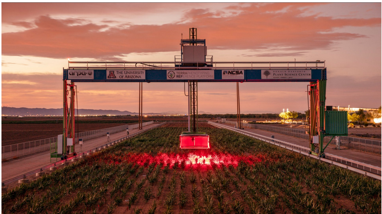
Rapid phenotyping gantry system with sensor array extended. Photo: Jesse Rieser for The Wall Street Journal.
